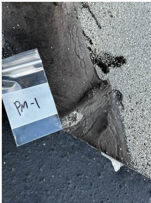
Picture 2: Penetration Mastic sampled from the exterior.
